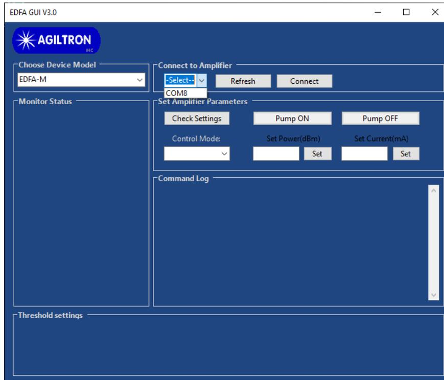
Figure 4: Remote control software: COM port selection.
