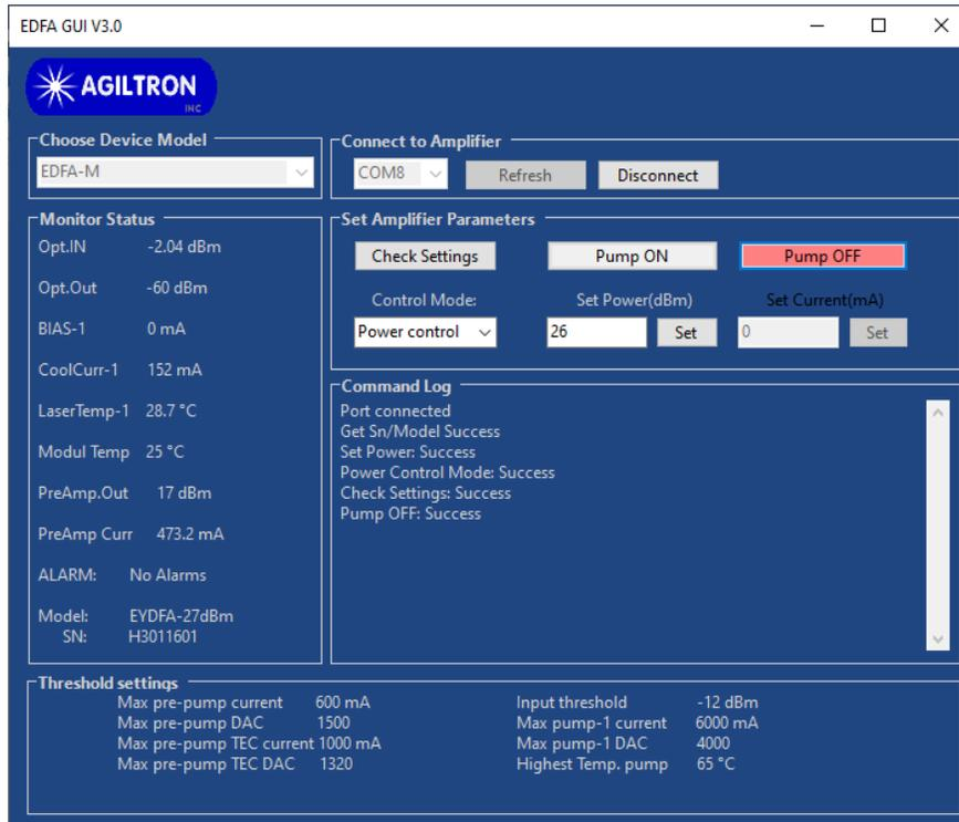
Figure 6: Remote control software: output is turned off.
