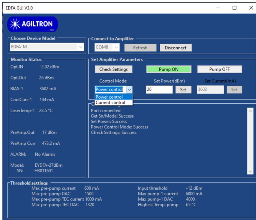
Figure 5: Remote control software: control mode selection
